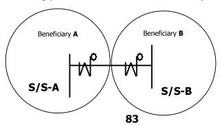
Net VArh exported from S/S-A, while voltage < 97% = X1Net VArh exported from S/S-A, while voltage > 103% = X2Net VArh imported at S/S-B, while voltage < 97% = X3Net VArh imported at S/S-B, while voltage > 103% = X4
