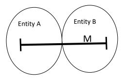
**Case- 2:** Interconnecting line owned by Entity – B Metering Point: Substation of Entity – A
