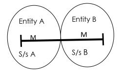
Net VArh exported from S/S-A, while voltage < 97% = X1 Net VArh exported from S/S-A, while voltage > 103% = X2 Net VArh imported at S/S-B, while voltage < 97% = X3 Net VArh imported at S/S-B, while voltage > 103% = X4
