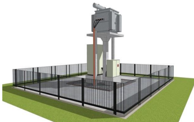
Plinth Mounted DT
