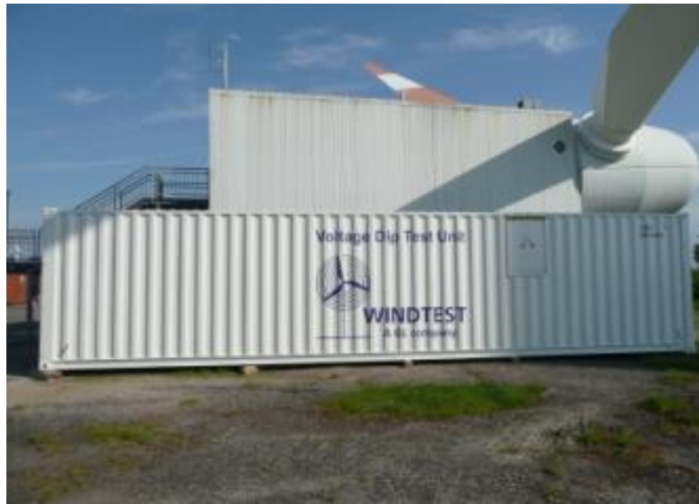
Figure 51: A turbine undergoing LVRT testing (source: DNV GL)
