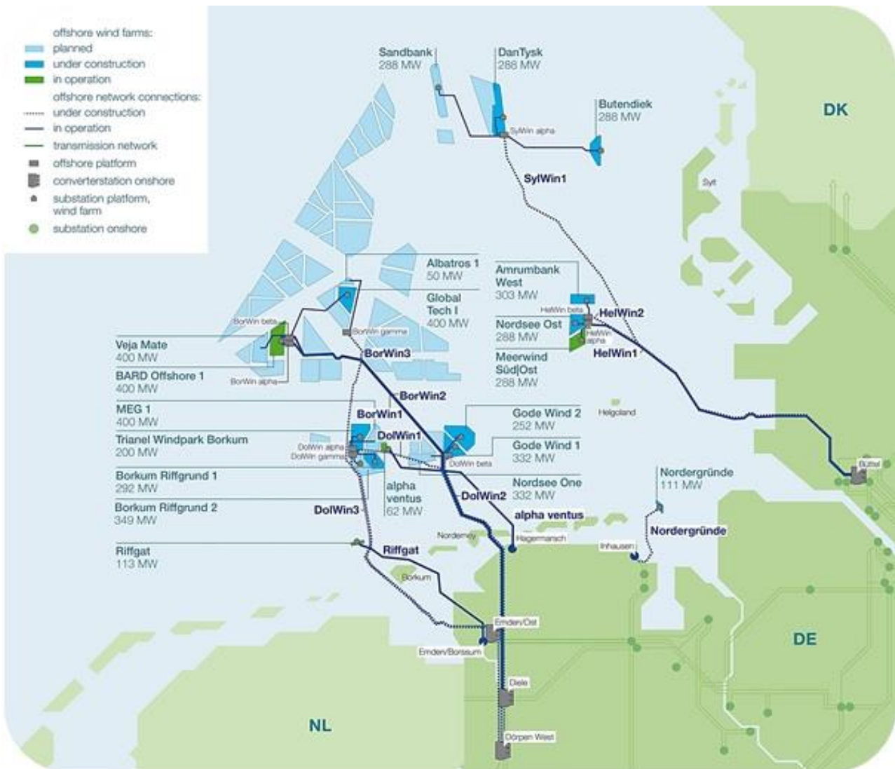
Figure 40: German North Sea Offshore Wind Farm Connections [34]
