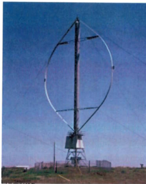
Fig-A22: Vertical Wind Axis Turbine
