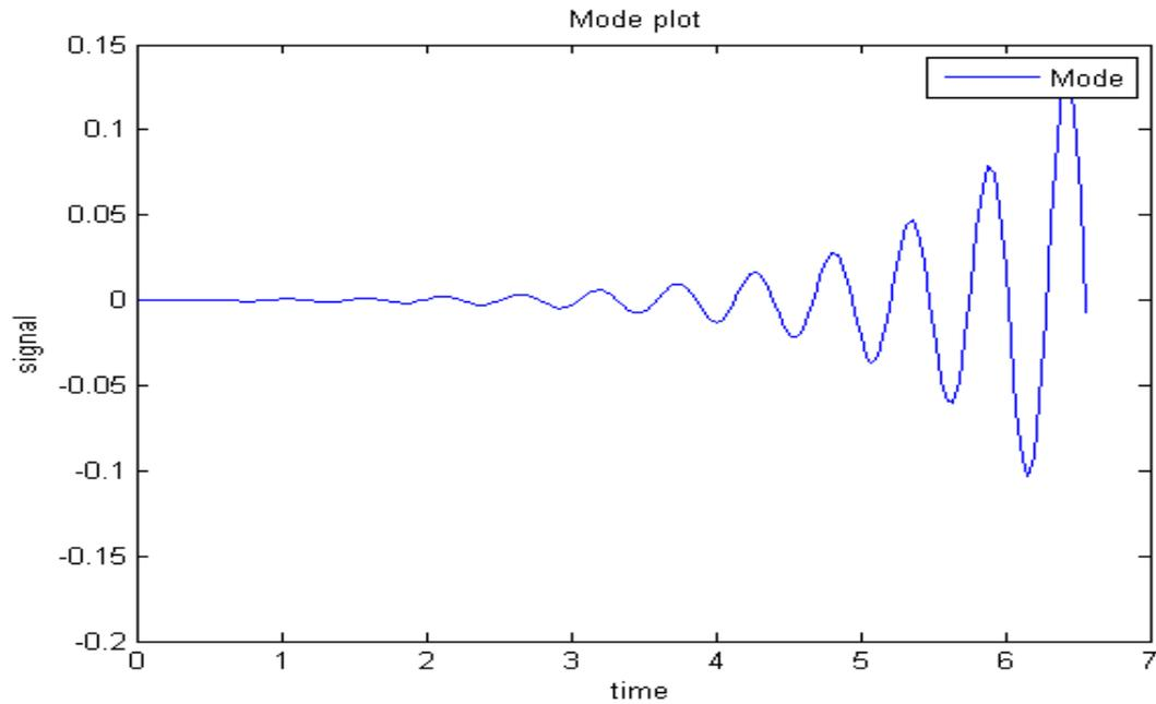
**Fig 6.5: 30<sup>th</sup> July 2012—1.85 Hz mode (damping -8.2%) during disturbance period**
