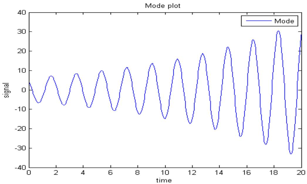
**Fig 6.7: 31<sup>st</sup> July 2012—0.53 Hz (damping:-2%)-pre-disturbance**
