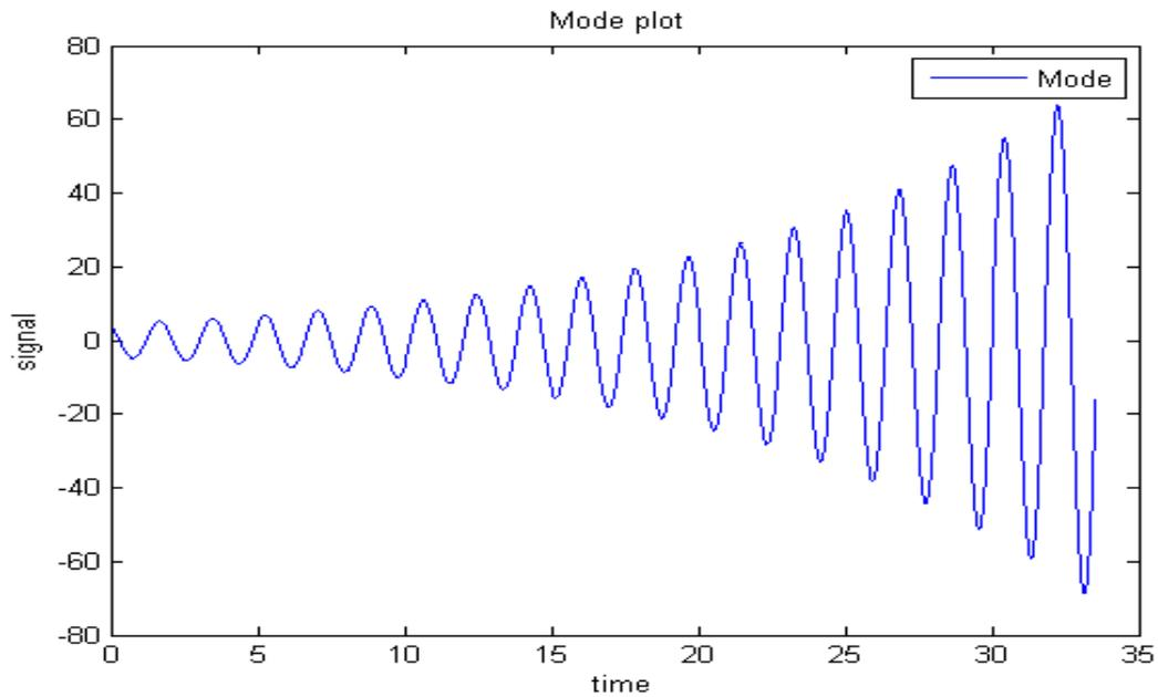
**Fig 6.7: 31<sup>st</sup> July 2012—0.55 Hz (damping:-2.3%)- disturbance**
