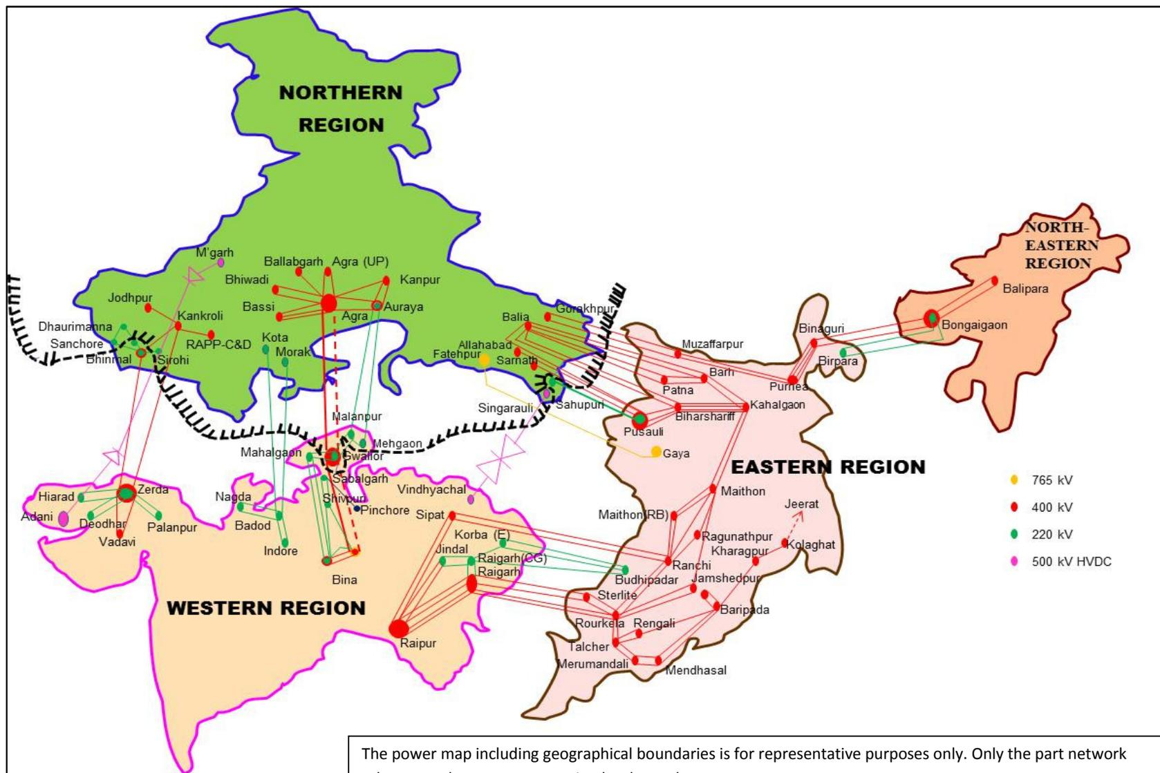
Figure 3.1: Sketch showing the axis of separation on 30<sup>th</sup> July 2012
