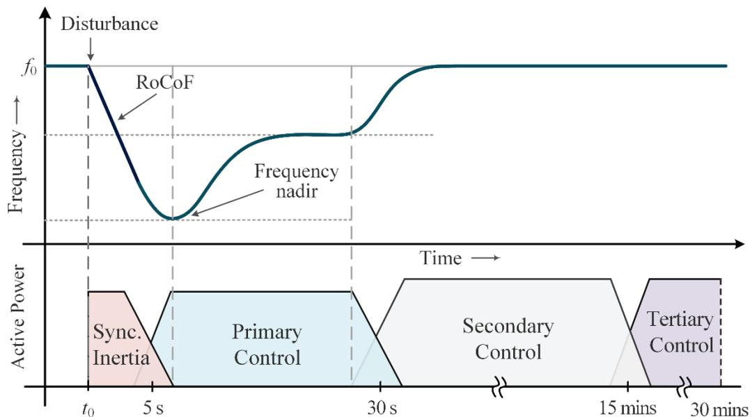
Figure 1.1 Stages of power system frequency response after a disturbance
