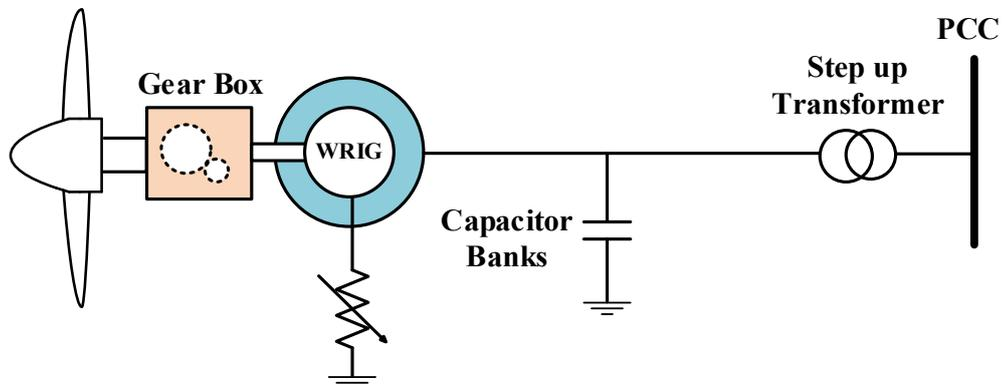
Figure 4.9 Variable-speed, wound rotor induction generator (Type-2 WTG)
