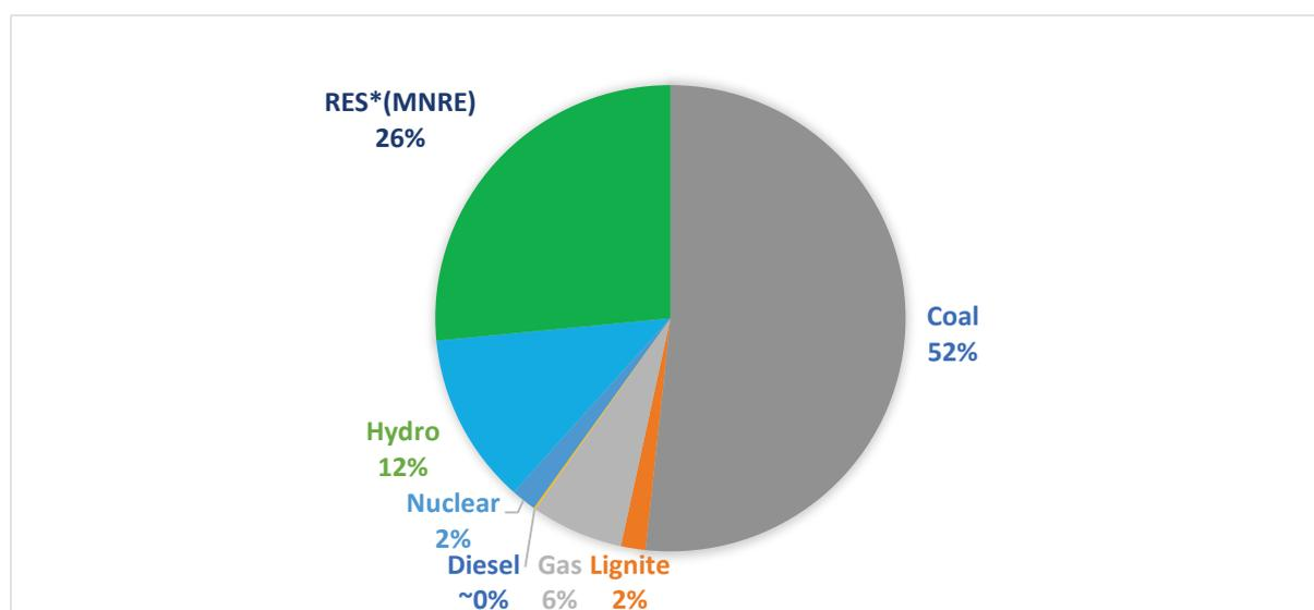
*Figure 4.1 Installed generation capacity in India*
