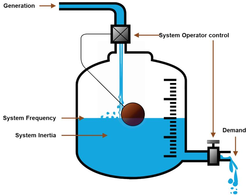
Figure 2.1 Power system inertia and water tank analogy
