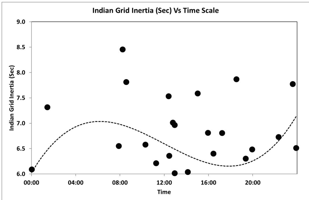
Figure 6.3 Grid Inertia vs Time of Day
