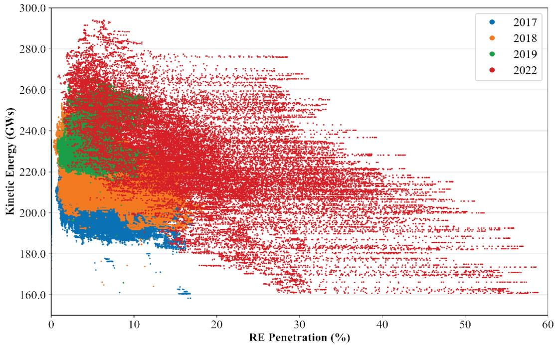
Figure 9.1 Variation of WR kinetic energy wrt RE Penetration
