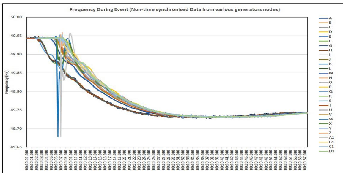
Figure 5.5 Typical time synchronization issues in high resolution frequency data
