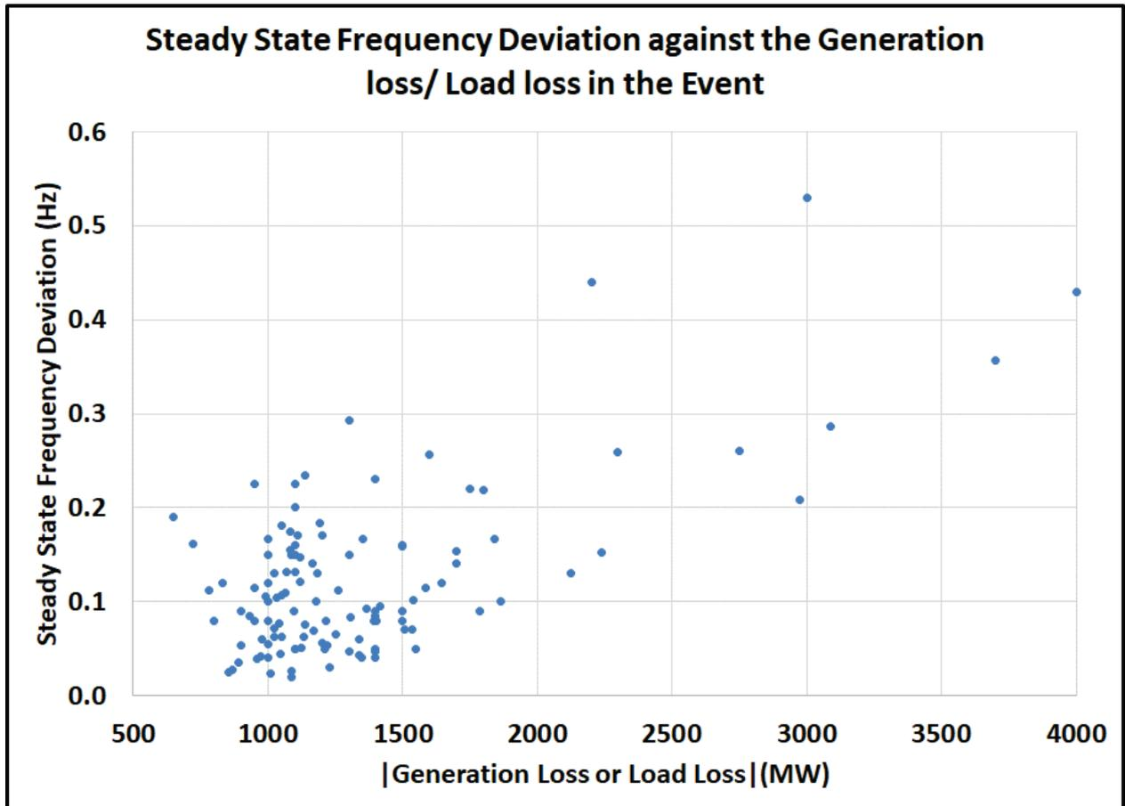
Figure 8.5 Magnitude of steady state frequency deviation against the event generation/load loss
