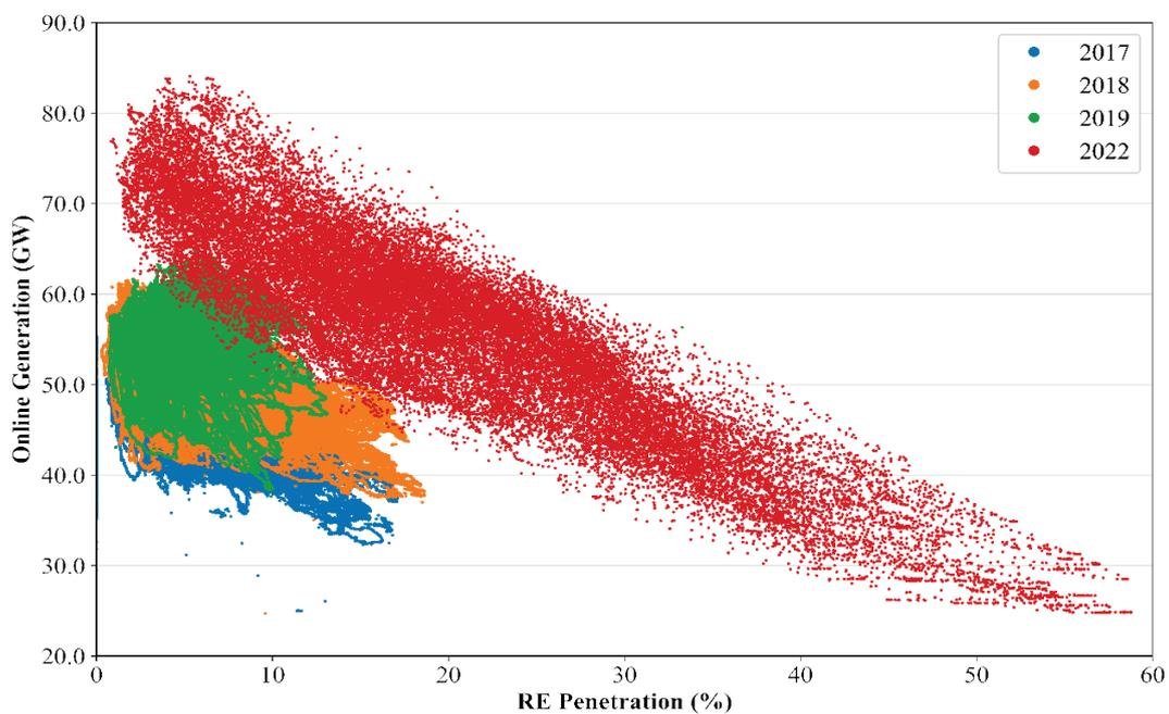
Figure 9.5 Synchronous generation of Western Region wrt RE penetration
