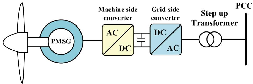
Figure 4.11 Variable-speed, permanent magnet synchronous generator (Type-4 WTG)
