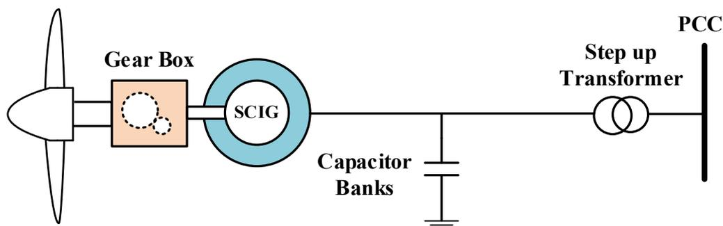
Figure 4.8 Fixed-speed, squirrel cage induction generator (Type-1 WTG)
