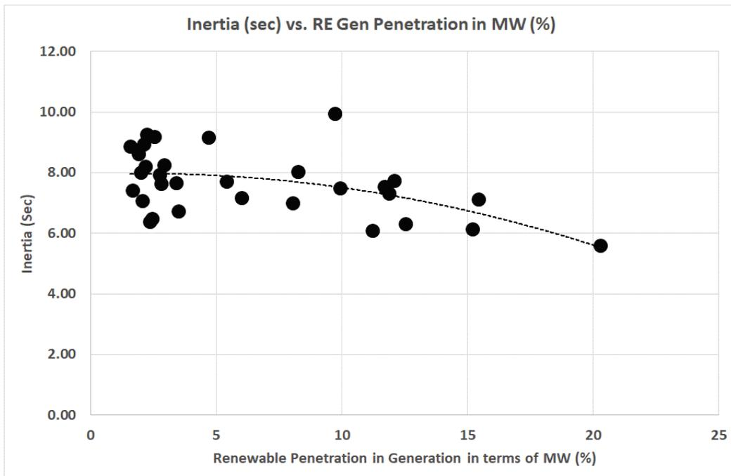
Figure 6.4 RE Penetration Vs Grid Inertia
