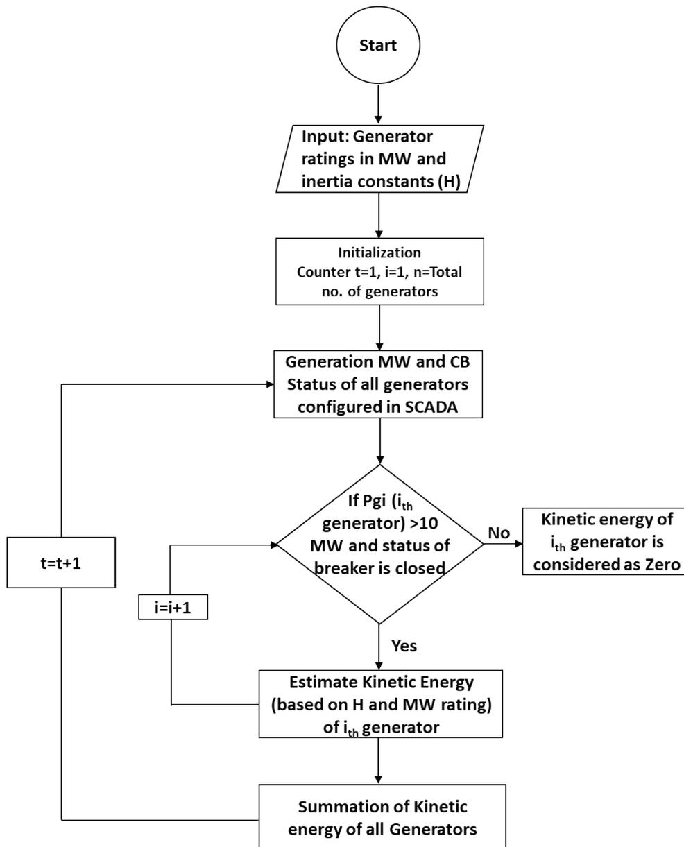
Figure 7.1 Flow chart for online inertia estimation
