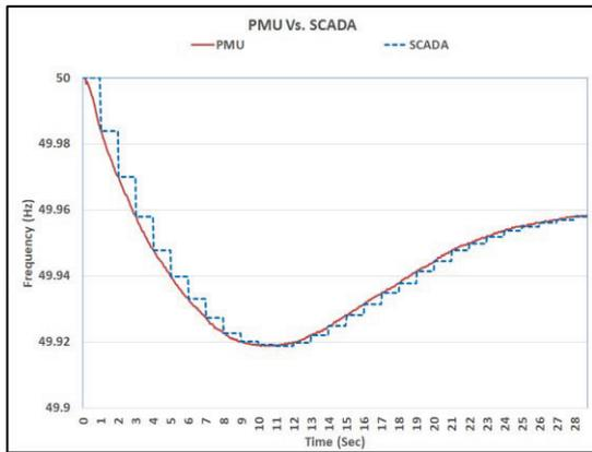
Figure 5.6 Frequency from PMU and SCADA for the same event
