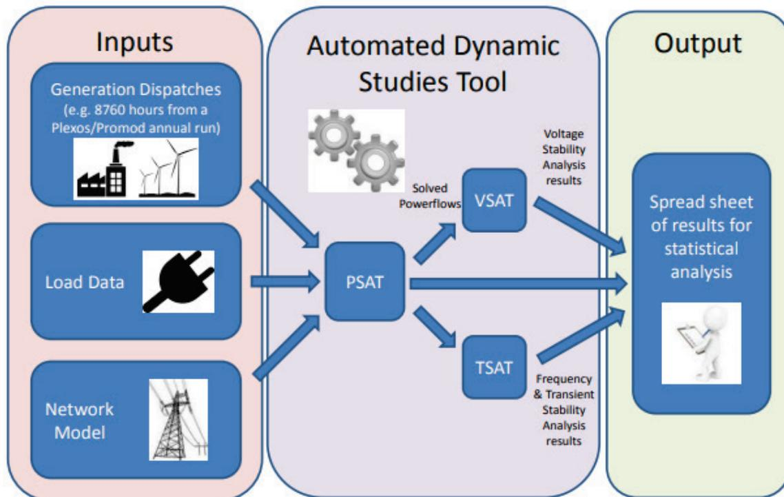
Figure 3.3 Overview of the Automated Dynamic Study tool process
