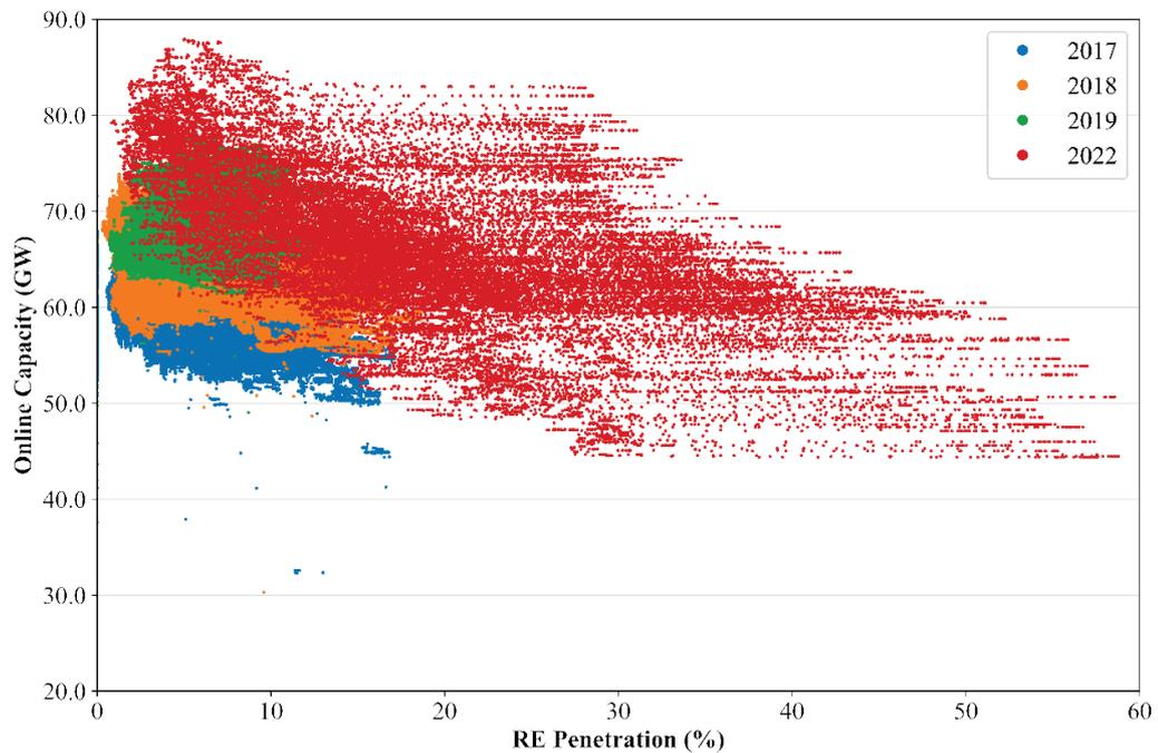
Figure 9.4 Online synchronous capacity of Western Region wrt RE penetration
