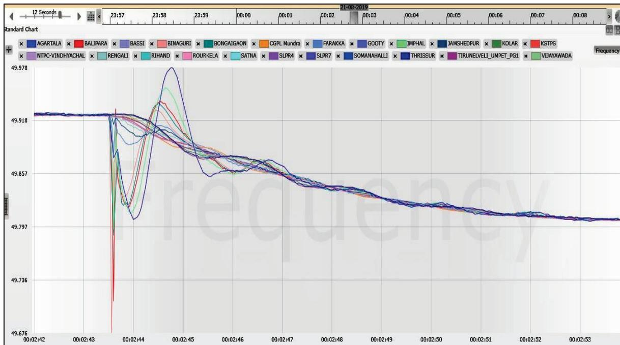
Figure 8.1 Frequency behaviour at different locations across the grid for generation loss event
