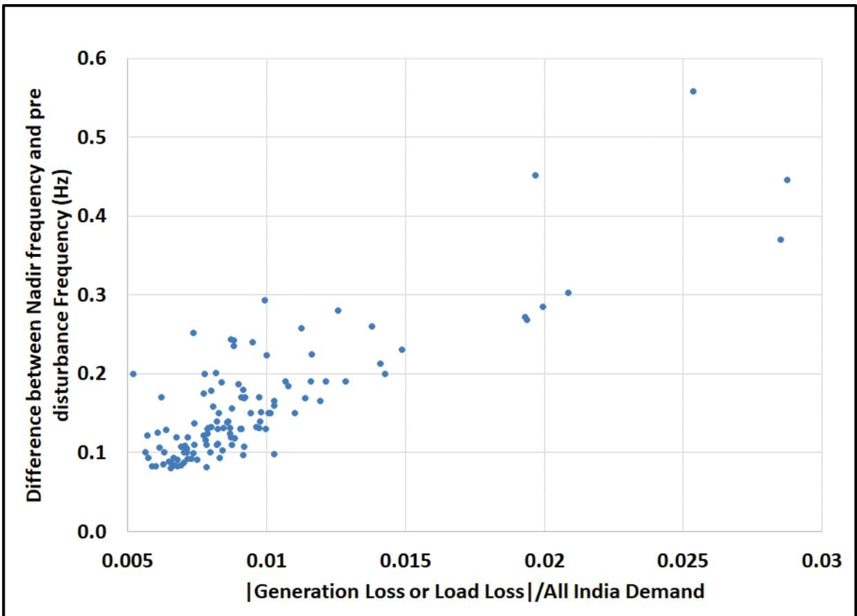
Figure 8.3 Maximum frequency deviation vs. normalized power imbalance
