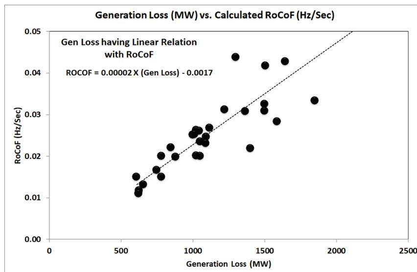
Figure 6.5 Generation Loss vs. Frequency Drop
