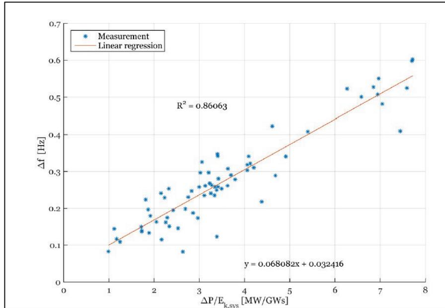
Figure 3.2 Maximum frequency deviation relative to power imbalance and estimated kinetic energy
