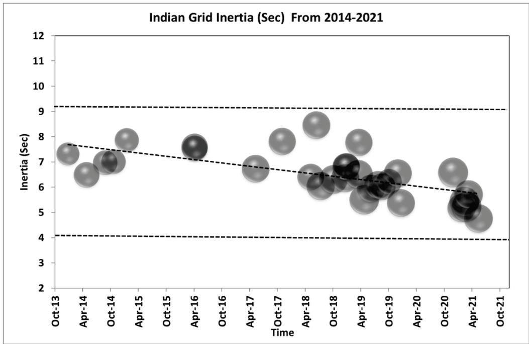
Figure 6.2 Grid Inertia on Year Scale
