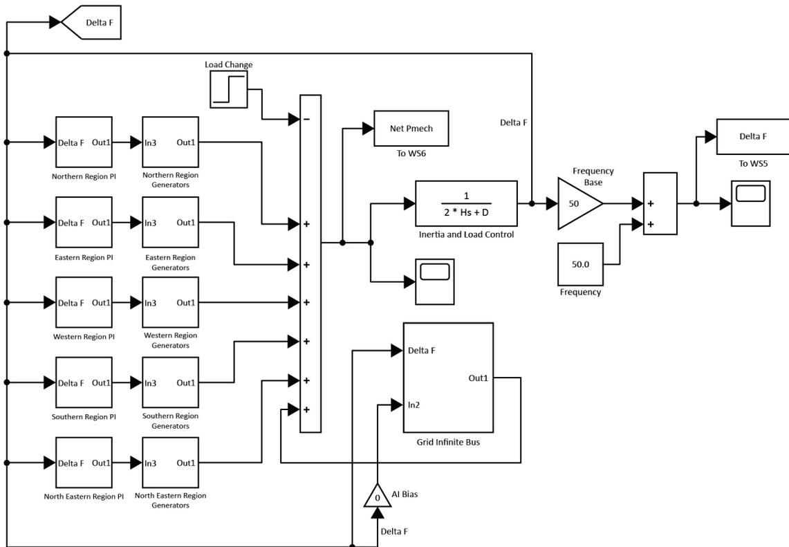
Figure 9.8 Multi-Region integrated Frequency Control model
