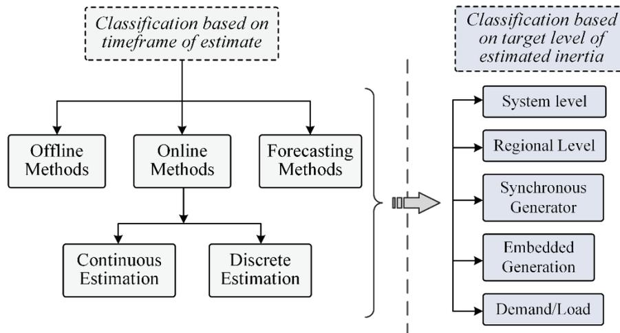
Figure 2.6 Classification of inertia estimation methods
