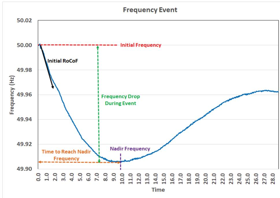
Figure 5.4 Approximate frequency response and other parameters of centre of inertia
