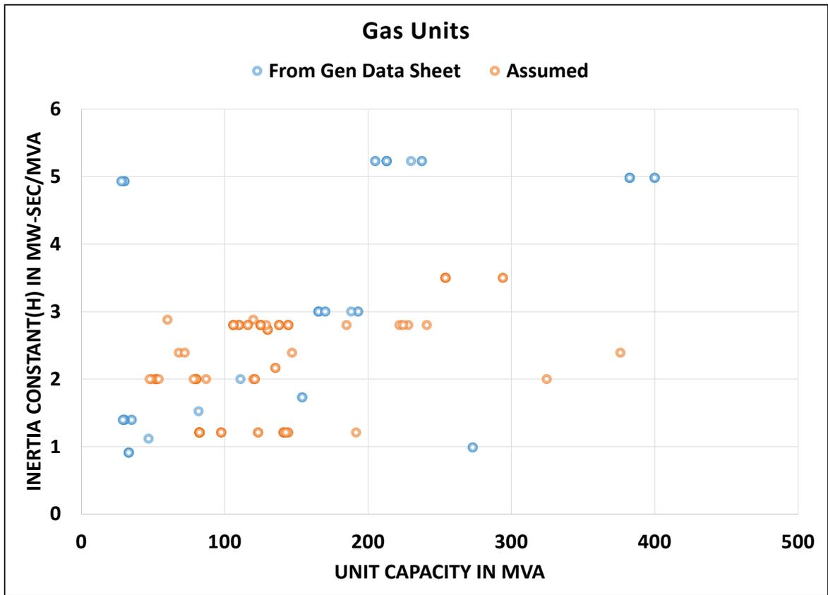
Figure 4.4 Inertia constant of Gas Generators in India
