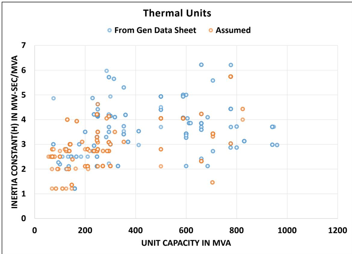
Figure 4.2 Inertia constant of Thermal Generators in India
