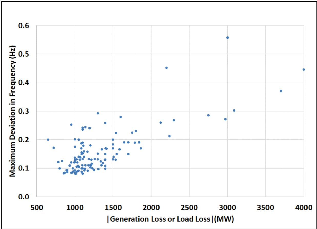
Figure 8.2 Maximum frequency deviation vs. power imbalance
