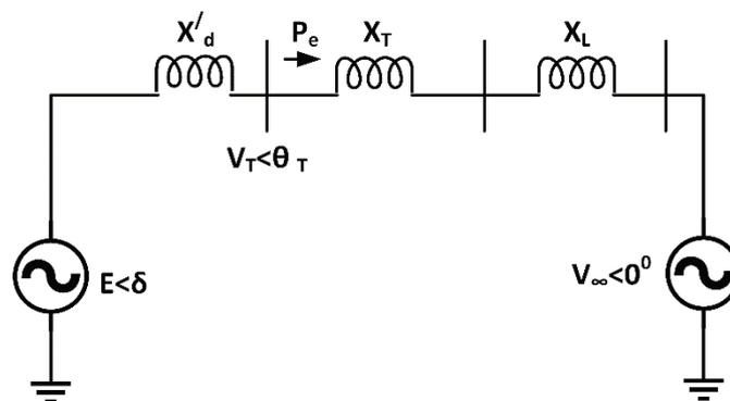
Figure 2.2 Impedance diagram of the single machine infinite bus system
