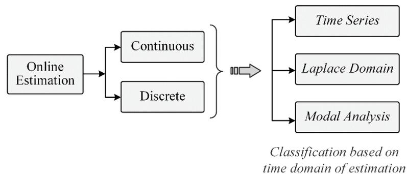
Figure 2.7 Sub classification of online inertia estimation methods
