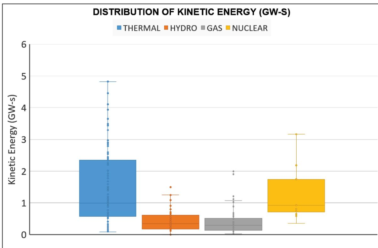
Figure 4.7 Box and Whiskers plot of Inertia constant of generators in India
