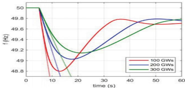
Figure 2.4 Impact of diminishing inertia on system frequency response [2]
