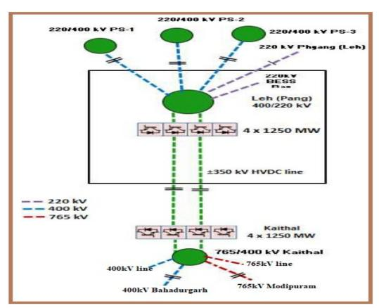
**2.5.** Regarding the query on type of cable being proposed and the losses in the HVDC system, CTU clarified that the 15 km underground cable proposed in the DPR is with XLPE cable. Further, the losses in HVDC system is around 6-7% (2% as HVDC terminal losses and 4-5% loss in HVDC transmission line). The conductor design has been proposed as Quad Lapwing considering the ±350 kV voltage.
