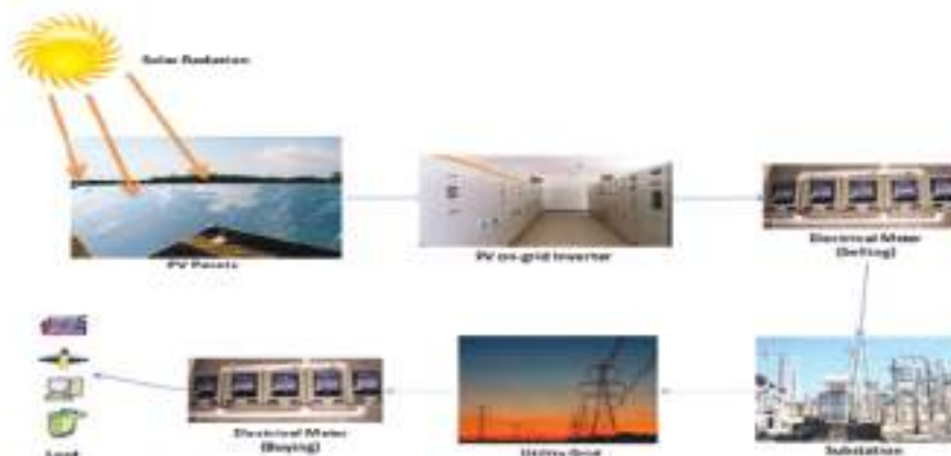
Fig-A.9 : Grid Connectivity of Solar Power Farms
