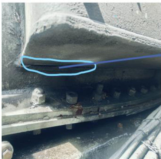
Damage and Oil spilling point
