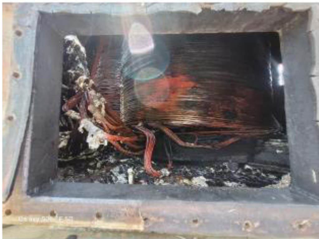
HV side winding (completely burnt)
