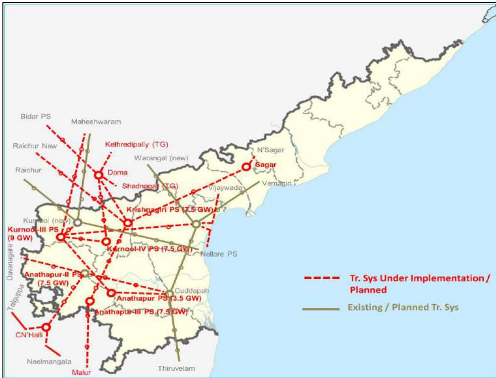
Fig.7: Transmission system for evacuation of RE power in Andhra Pradesh
