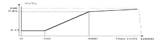
Provided that during the voltage dip, the supply of reactive power has first priority, while the supply of active power has second priority and the active power preferably be maintained during voltage drops, provided, a reduction in active power within the plant's design specifications is acceptable and active power be restored to at least 90% of the pre-fault level within 1 sec of restoration of voltage.
